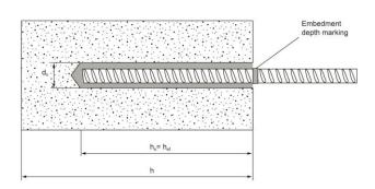
Table A2: Installation details for rebar
