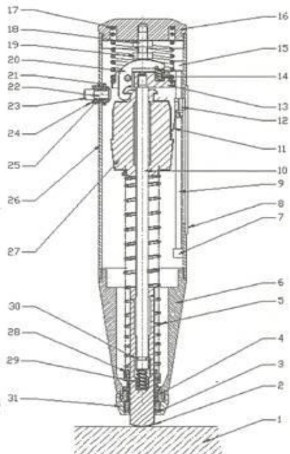
Figure 1 Structure of Test Hammer HT225
