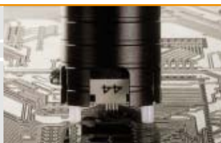
SR-SCOPE® RMP30-S: Cu on printed circuit board
