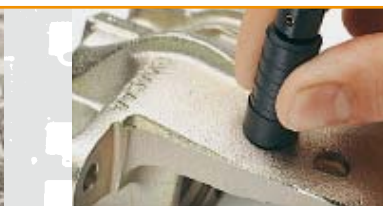
PHASCOPE® PMP10: Zn/Fe with a rough surface
