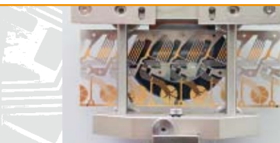
Sensor contacts: Au/Ni/CuFe
