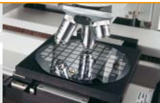
Wafer: Hardness determination on the gold coating
