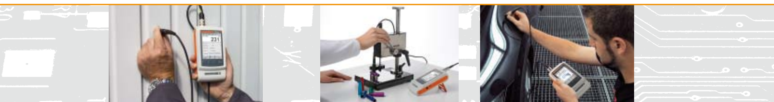
Measuring paint coating on steel
